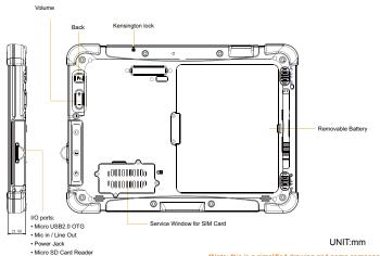
\*Note: this is a simplified drawing and some components are not marked in detail. Please contact our sales representative if you need further product information. \*\*Note: Measured at dimning LCD brightness. Varies depending on the usage conditions, or when an external device is attached.
